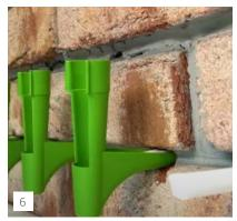
Insert the end of the capillary rod into the suction angles' supply tank and then push the capillary rod and the suction angle together into the drill hole so that the suction angle is securely stuck in the hole. The suction angle is reusable. The KÖSTER Capillary rods are not prewetted.
